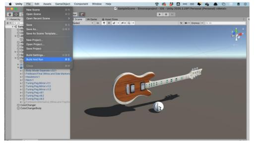
In order to deploy the application, the latest version of Unity and Xcode will need to be installed on the hard drive of the operating system of the device. When the next version of the application is ready to be deployed and you will have to go File>Build and Run.
